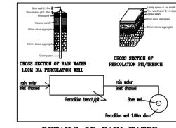
DETAILS OF RAIN WATER HARVESTING STRUCTURES
